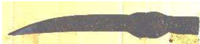
Illustration 1 Rust sludge remains on object surface after electrolysis
