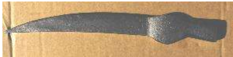
Illustration 2 Clean steel surface after sludge has been brushed off
